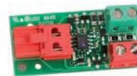
BUS XIB interface (for E045 or E045S or E024S boards with photocell no BUS)
