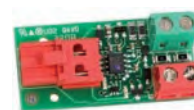
BUS XIB interface (for E045 or E045S or E024S boards with photocell no BUS) 790062
