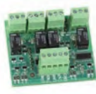
I/O expansion card - 4 OUTPUT 24VDC 1A - 4 INPUT
